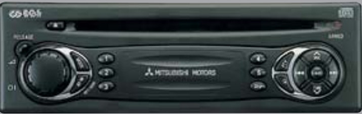
PH-3850 Radio/CD player with RDS-EON tuner, CD changer control buttons, trip computer mode switch, telephone mute preparation and detachable front panel, 4 x 40W. Standard equipped with Jazz Black front panel. MZ312637
